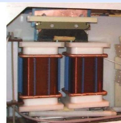
Figure 6. 330 kW Nanocrystalline Boost Transformer
